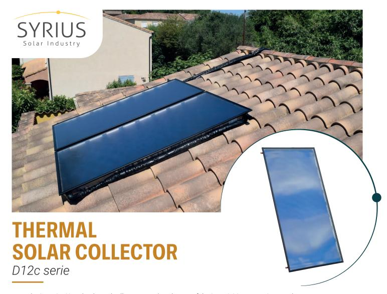
The SYRIUS D12c solar thermal collectors complete the core of the SYRIUS SOLAR INDUSTRY product range. They combine the strengths of the D12 series with a new generation of absorbing surface to limit overheating. Just as efficient as its counterpart in normal Functioning, this new coating increases its emissivity at high temperatures, which significantly reduces the stagnation temperature.
